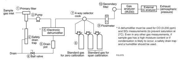
Measurement of sample gas with high moisture content or NO, SO<sub>2</sub>, or CO (0-200 ppm range) measurement
