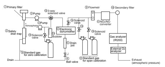
\*A dehumidifier must be used for NO, SO<sub>2</sub>, and CO (0-200 ppm) measurements (to prevent saturation at 2°C). Use either atmospheric air or cylinder gas as a zero calibration gas and supply it through a bubbler (humidifying) to reduce interference of water.
