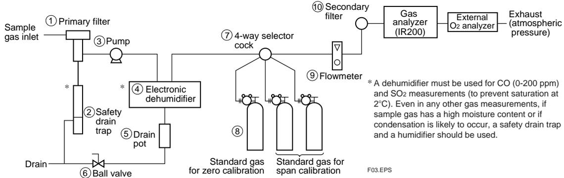
Measurement of sample gas with high moisture content or NO, SO<sub>2</sub>, or CO (0-200 ppm range) measurement
