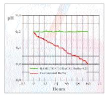
A complete range of patented buffer solutions provides never before achieved pH stability. HAMILTON guarantees DURACAL pH buffers for 5 years after the date of manufacture. The pH 9.21 and pH 10.01 buffers are even stable in air. See the diagram for details. High buffering capacity provides rapid stable calibration. Preservatives are added to prevent microbial and mold growth.
