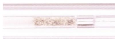
EVEREF-F system contains a silver barrier which prolongs electrode life in aggressive samples.
