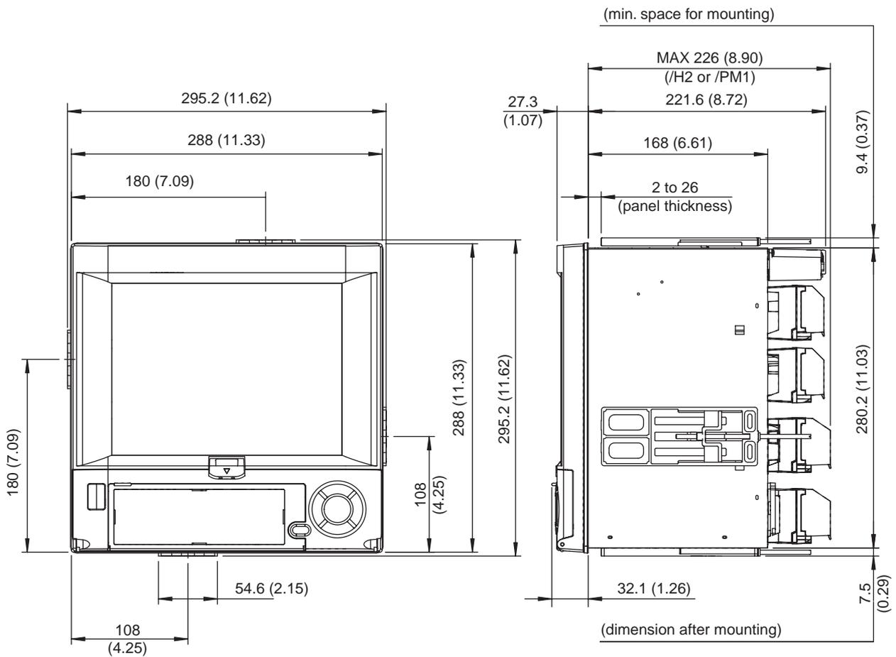
Note: If not specified, the tolerance is  $\pm 3\%$ . However, for dimensions less than 10mm, the tolerance is  $\pm 0.3\text{mm}$ .
